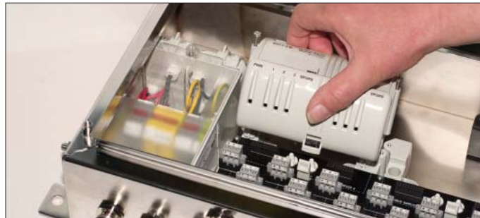
Figure 5.1 - Fieldbus Barrier module - fitting & removal
